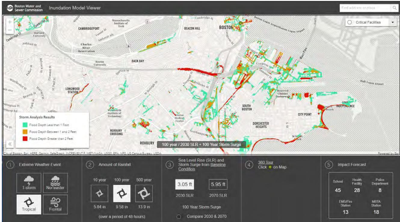
**For the Boston Water and Sewer Commission ([bwsc.org](http://bwsc.org)),** Hazen used existing 1D hydraulic models as a starting point to develop a 2D model that predicts flooding from varied coastal and rain events throughout the city. GIS tools assessed impacts and vulnerabilities to critical infrastructure resulting from
